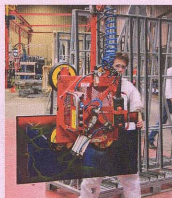
GLASS IS MOVED BY HAND OR WITH AN AIR-POWERED LIFTING CRANE.
